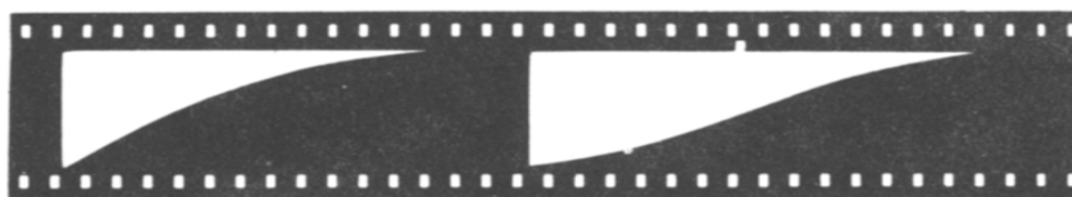
Fig. 2. Typical gradient functions photographed on 35 mm film. Note that the buffer vessel change-over cue spot is displaced from the function change by a distance equal to that between the scanning slit and phototransistor hole (3.5 cm in our instrument).
